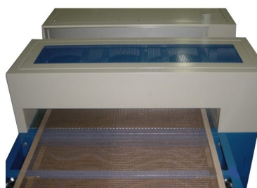
Possibility to have air cooling bridges to low temperature from textile in exit
