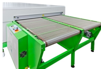
Possibility to build dryer with 2 belt systems
