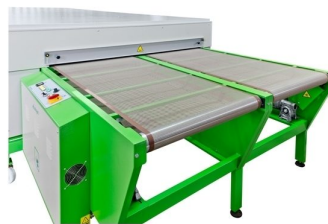
Possibility to build dryer with 2 belt systems
