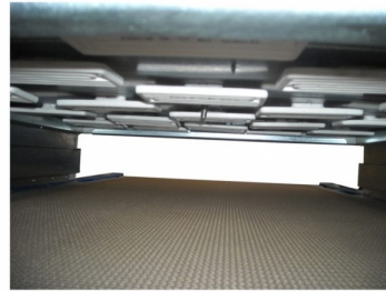
Perfect heating distribution in belt width direction to have perfect drying results
