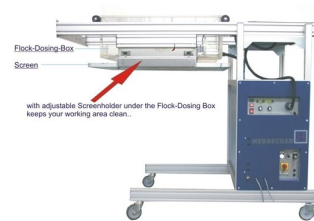
Flocking stations available for manual or automatic printing machines
