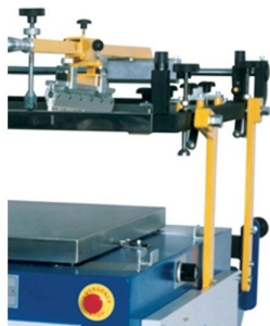
Screen printing frame allways in horizontal position
