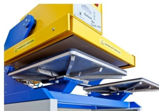
Bottom plates with free arm and with possibility to change sizes
