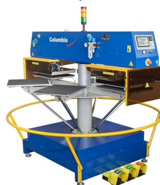
Bottom plates with free arm and with possibility to change sizes
