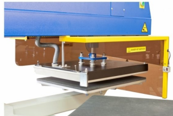
Security photocell for operator safety
