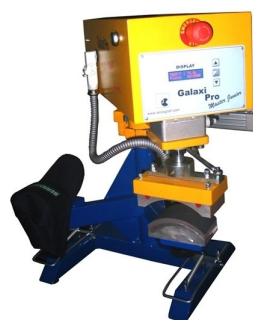
125 mm pressing cylinder course so you can transfer in high profile pieces
