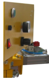
Side movment made by pneumatic cylinder
