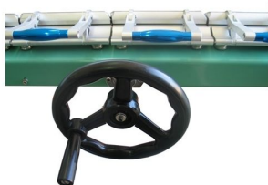
Adjusting from mesh tension made with smoothness and accurate values
