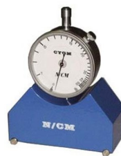
Tensiometers to check mesh tension available
