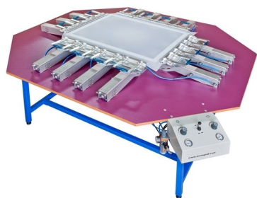
Mesh stretcher with pneumatic clamps available
