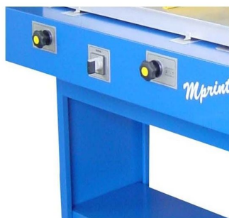
Micrometric registers on the printing plate
