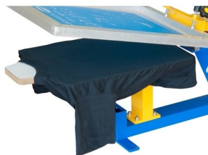
Off contact in printing station
