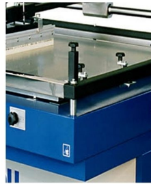
Possibility to print in flat material with height up to 100 mm
