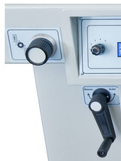
Printing table can be adjust in height up to 20 mm by using a handle
