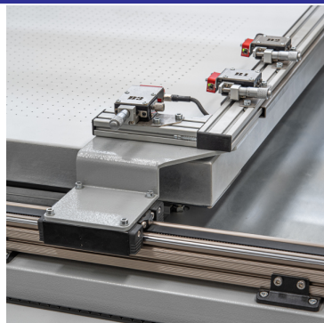
3 Photocell for printing marks reading
