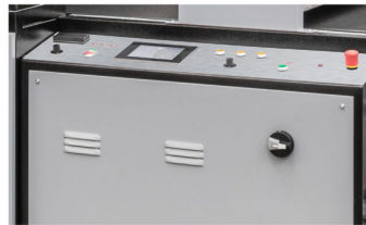
Control panel with 7 inches touch screen
