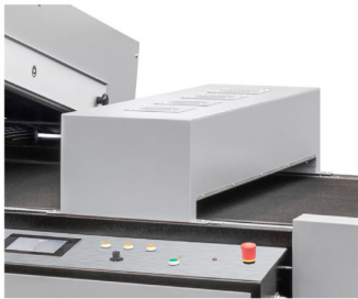
3xIR lamp box with power adjustment between 20% to 100%
