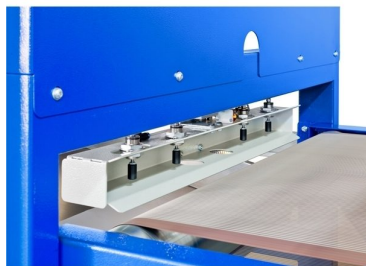
Gripping clamp equipped with 4 pressure cylinders with position adjustment
