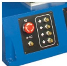
Print speed and stroke, flood speed and stroke with individual adjustments
