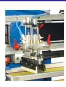
Printing/Flood angle and force with individual adjustment
