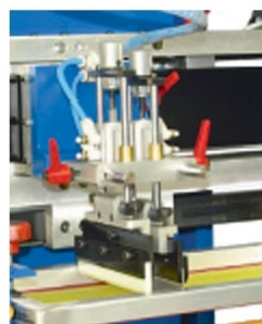
Printing/Flood angle and force with individual adjustment
