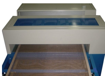
Hot air turbine with re circulation from air in closed circuit for option water base drying
