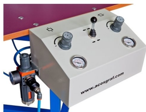
Stretching pressure with individual adjustment in both XX and YY axes
