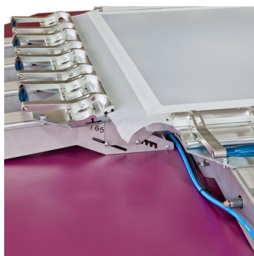
Possibility to adjust for several screens heights with toolless operation
