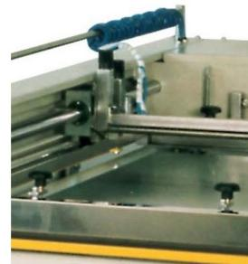
Individual adjustment from pressure and inclination angle for flood bar and squeegee
