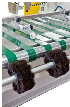
Brush systems in the entry from stacker to have a perfect sheet transport
