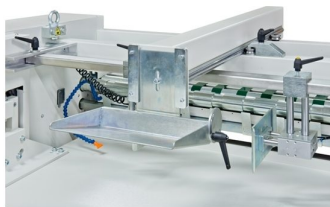
Tool less system to make all necessary adjustments from sheet stacking
