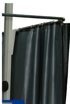
UV curtain to protect operator from UV light exposure
