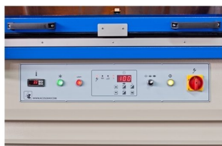
LCD control panel equipped with photocell from light intensity measure to make automatic compensation from
