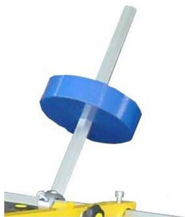
Counter weight with position adjustment to achieved perfect balance from screen
