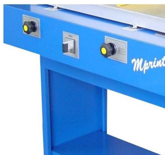
Micrometrics registers on the printing plate
