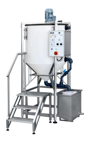
The OSCAR 500 is wastewater treatment plant used in screen printing. The OSCAR 500 can remove all debris from the water used in screen printing to: wash; developing, stripping, cleaning, etc... The OSCAR 500 is equipped with a 2-stage water treatment system: removal of solid particles and cleaning of color pigment.
