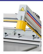
Emergency security bar withautomatic reverse fromdescending to ensure operatorsafety in all machine area
