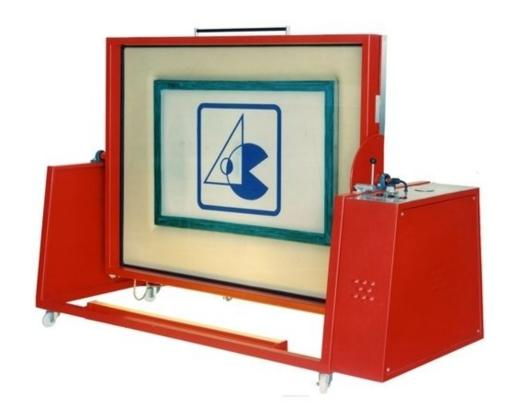
The VERTSCREEN is a machine suitable to make the vacuum and make the contact between screen and film. The VERTSCREEN has the possibility to rotate the screen to 180 degrees so you can insolate the screen in vertical position. The VERTSCREEN can be equipped together with the halogen lamp LUX RAPID and also with the ACOSGRAF electronic board with photocell from light intensity measure to make automatic compensation from exposure times.
