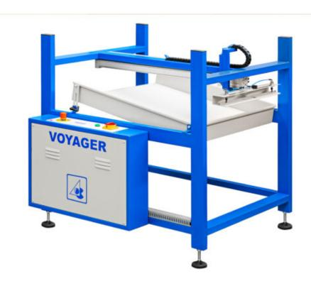
The VOYAGER automatic stacker that makes the collection from the printing sheet the exit of the tunnel using a pneumatic clamp. The stacker VOYAGER is available in different designs and can be used individually or integrated into printing lines. The VOYAGER can be equipped with one or two individual clamps for sheet retreat from dryer.
