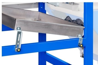
Reception table with inclination and height adjustment possibility
