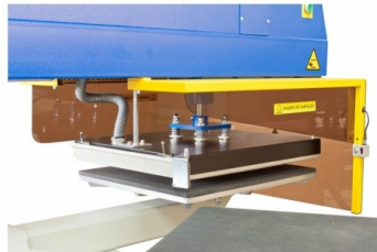
Security photocell for operator safety
