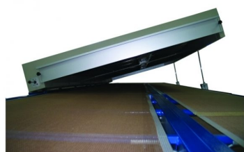
Possibility to equiped dryer with 2 belt systems
