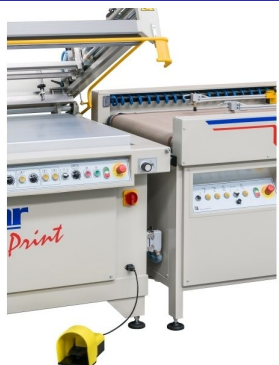
Lateral removal from sheet can be left or right position
